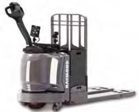
» With the Extreme Environment Corrosion Package, our trucks withstand the harshest applications, including food processing and harsh, caustic wash downs.
