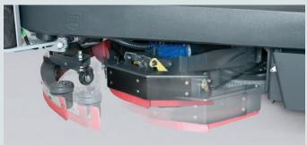
Retractable 4 inch (10 cm) offset disc deck enhances edge scrubbing and resists damage from accidental impact.
