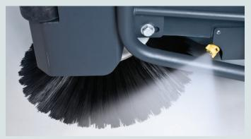
Patented DustGuard<sup>™</sup> is proven to reduce airborne dust generated by side broom sweeping. An ultra fine fog suppresses fugitive dust.
