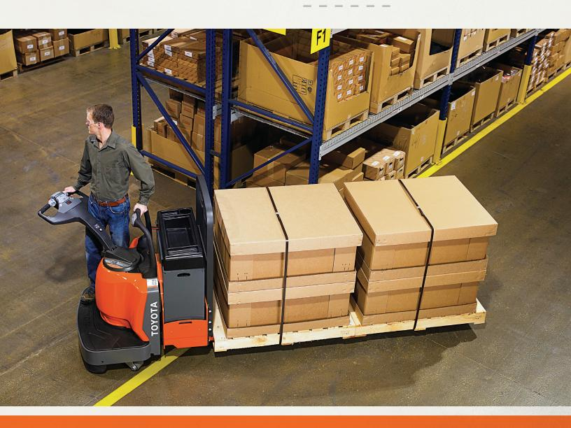
**FORK SIZE RANGE** CAPACITY 6000 - 8000 LBS. 36 - 144 IN. INDUSTRIES Food Storage Beverage Cold Storage \* STANDARD FEATURES PERFORMANCE • AC drive motor with thermal protection Adjustable maximum speed & current limiting Adjustable acceleration • 24-Volt electrical system On/off kev switch • 6" lift Lift limit switch
